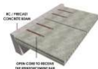
Lightweight concrete hollow core wall / floor panel
